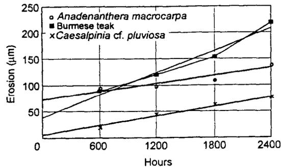
FIG. 1. Erosion of *Anadenanthera macrocarpa*, *Caesalpinia cf. pluviosa* (momoqui), and Burmese teak versus time of exposure in a weathering chamber (xenon arc radiation and periodic water spray). Each point is an average of 18 observations.
